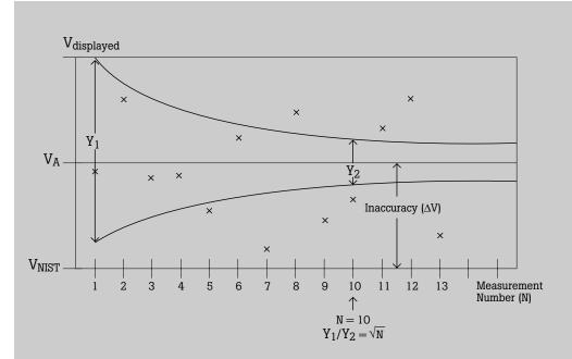
The effect of averaging readings in order to reduce noise in measurements.
